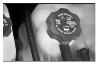
The coolant surge tank and pressure cap are located on the driver's side of the vehicle, toward the rear of the engine compartment. See *Engine Compartment Overview on page 356* for more information on location.
